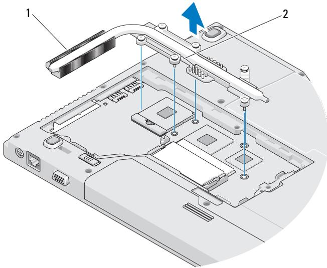
1 processor thermal-cooling assembly
